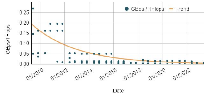
Ratio of I/O bandwidth (GBps) / TFlops of the top 3 of the Top500
