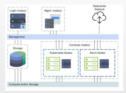
Setup: Partition K8s and Slurm nodes.<sup>1</sup>
